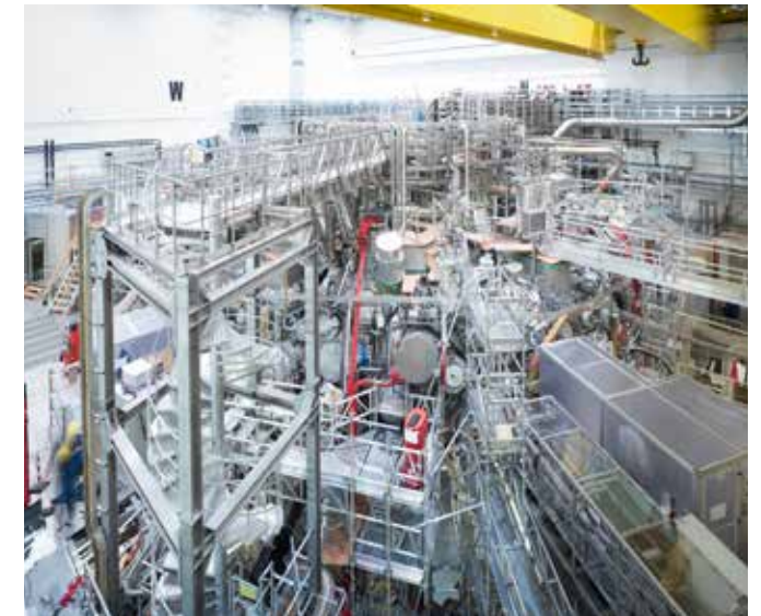
Wendelstein 7-X has a diameter of 16 m and a total weight of about 1000 t. Photo: IPP, J. Hosan
